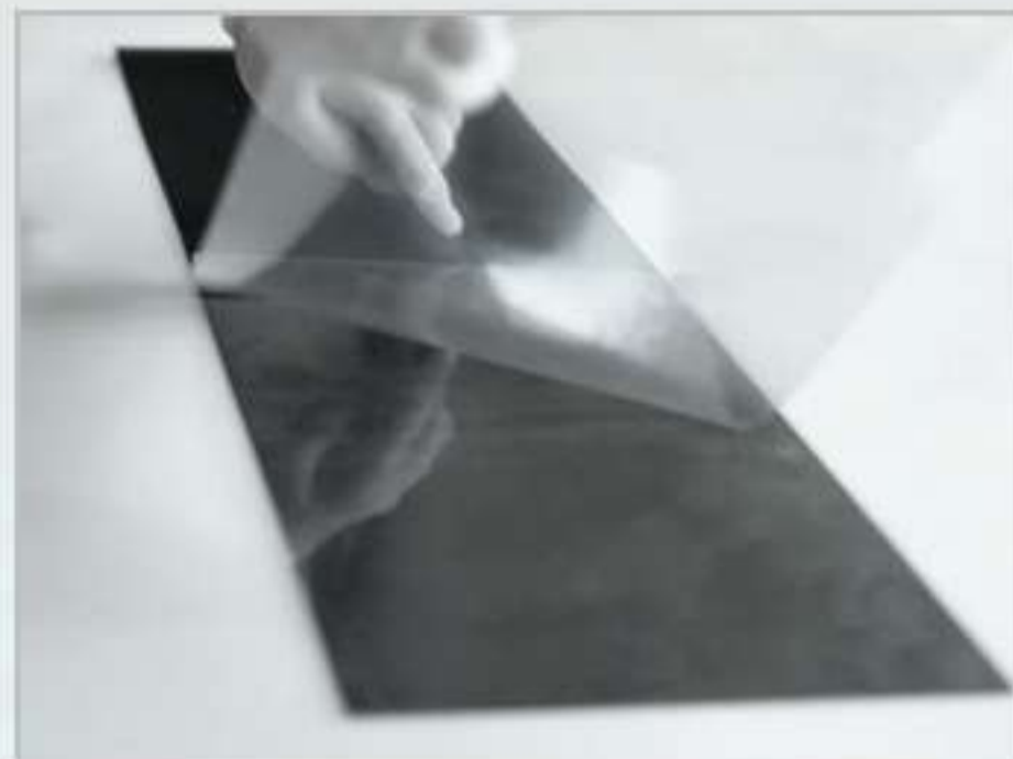
Step 3. Remove the protective film from the module back.
