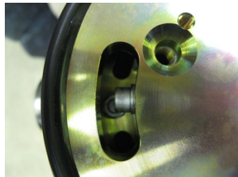
Fig. 15: Limit screw alignment
