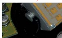
Radar module that is horizontally and vertically tiltable
